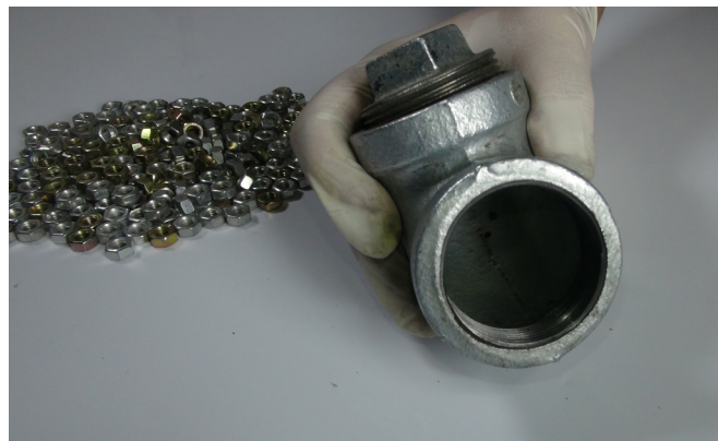
1. We will use a 1.5 inch metal elbow pipe, as shown above.
